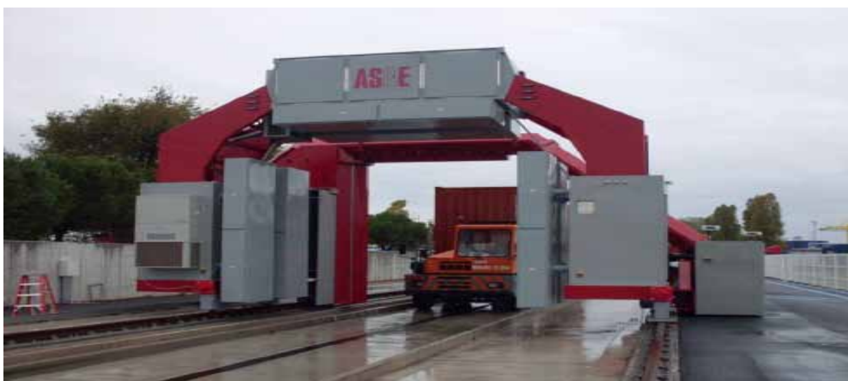
Scanner RX Omniview Gantry
